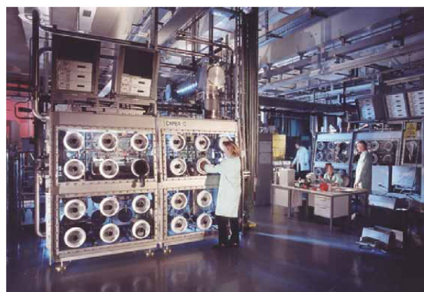
Fig. 2. The CAPER process (top) and facility (bottom) at the Tritium Laboratory Karlsruhe for the experimental demonstration of TEP systems, comprising as final clean-up a catalytic membrane reactor ( Q = H, D or T ).
