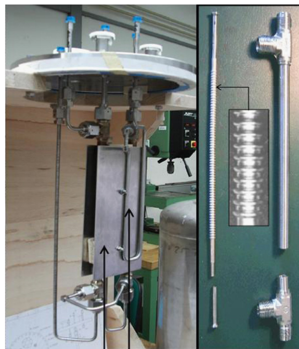
Fig. 6. View during manufacturing of a tritium compatible PERMCAT reactor mounted on a CF250 flange with 2 single-tube units in line (on the left) and the PERMCAT unit comprising a corrugated membrane (on the right).
